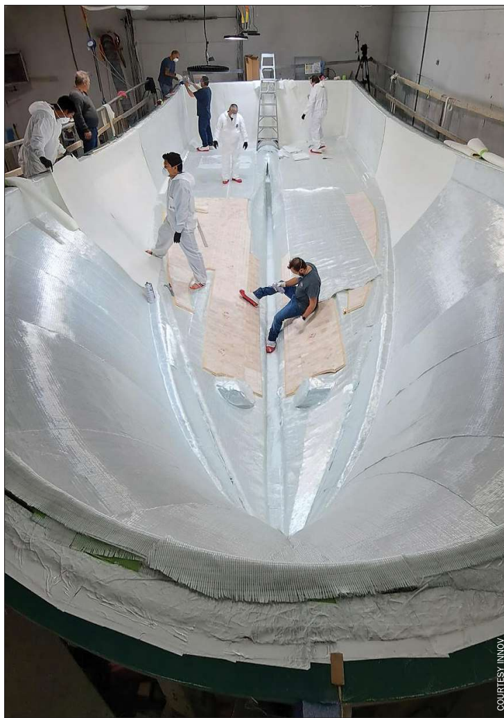
The team spent a week cutting laminates and loading the mold with layers of E-glass and some sheets of balsa core visible here on the bottom panels.
