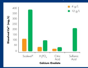
**Test conditions:** A cube of calcium carbonate (1 cm $^3$ ), or powdered calcium oxalate (6 g) was immersed in 100 g of acid solution (4 g/L or 12 g/L = 0.5 or 1.5 oz/gal) for 24 hours at 70°C (158°F).
