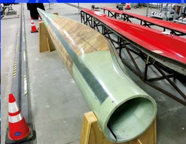
Arkema has developed a thermoplastic resin that means it is now possible to make fully recyclable wind turbine blades.
