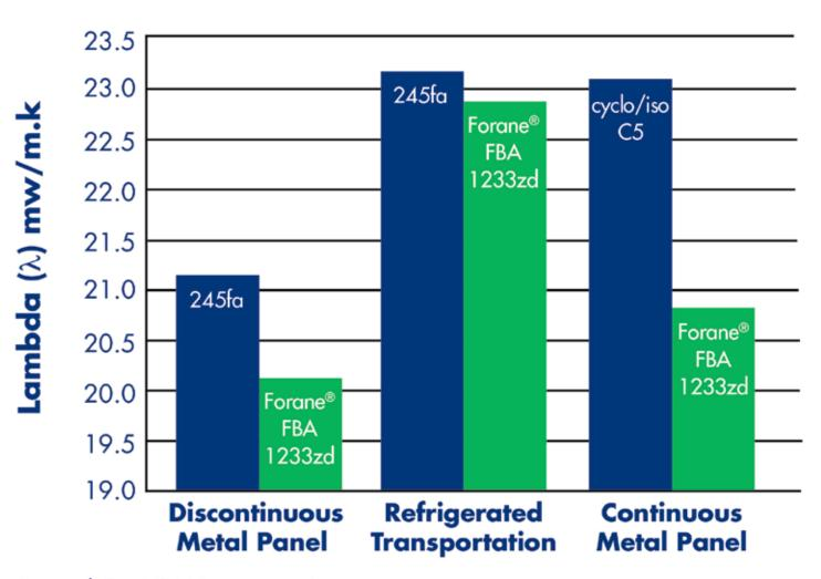
\*Tested @ 75°F Mean Test Temperature
