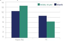
Formulation (phr): PVC Kw62: 100, tin maleate: 2.1, internal lubricant: 0.8, ESBO: 1, Plastistrength® 550 PA: 2, Plastistrength® L1000 PA: 0.15, oxidised PE wax: 0.15, IVA: 0.3
