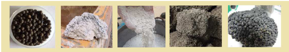
Figure 2: Impact on molecular sieve due to contaminants
