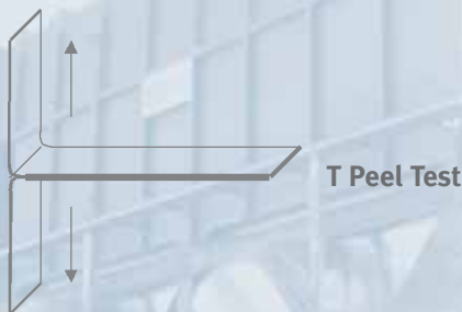
Bonding Aluminium to Aluminium: T Peel Test
