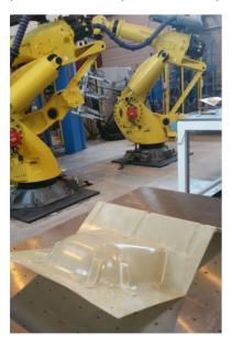
With the Elium<sup>®</sup> technology, Arkema offers a range of liquid thermoplastic resins processed by the same methods (resin transfer molding, infusion, flex-molding) as those used for thermoset resins, hence keeping down capital expenditure for processors.
